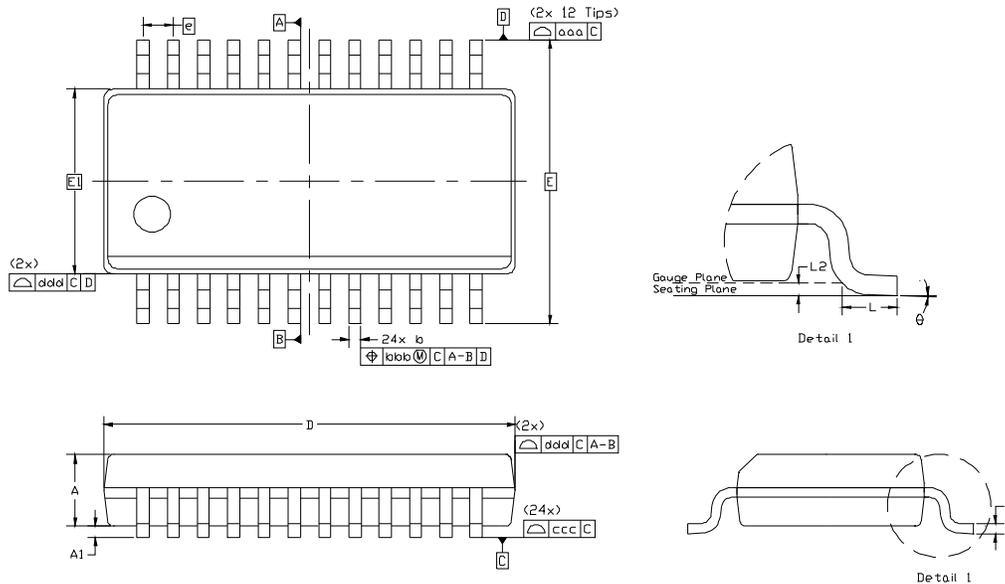
**Figure 13. 24-Pin SSOP**
